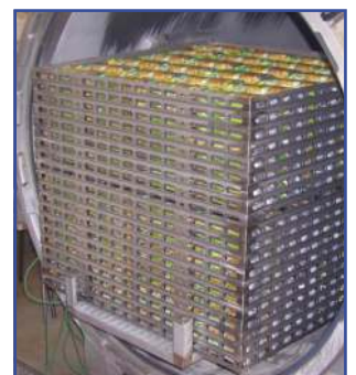
Käfiglos stapelbare Trays Cageless stackable trays
